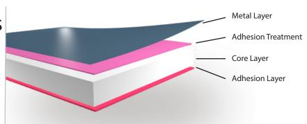
HIGH BARRIER METALLIZED PET FILM WITH VERY GOOD METAL ADHESION
