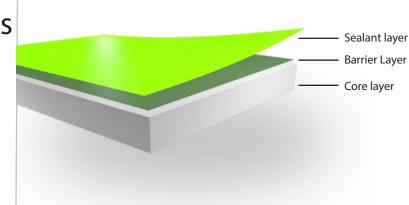
ULTRA HIGH BARRIER PEELABLE LIDDING FILM, SEALABLE TO MOST RIGID SURFACES
