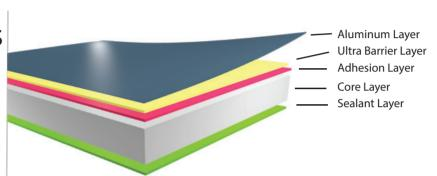
ONE SIDE HEAT SEALABLE, ONE SIDE METALLIZED HIGH BARRIER BOPP FILM
