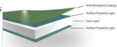
SUPER CLEAR UV STABILIZED THREE LAYER PET FILM, ONE SIDE PRINT RECEPTIVE COATING
