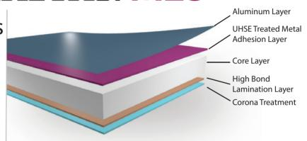
ONE SIDE TREATED, ONE SIDE METALLIZED NON SEALABLE BOPP FILM
